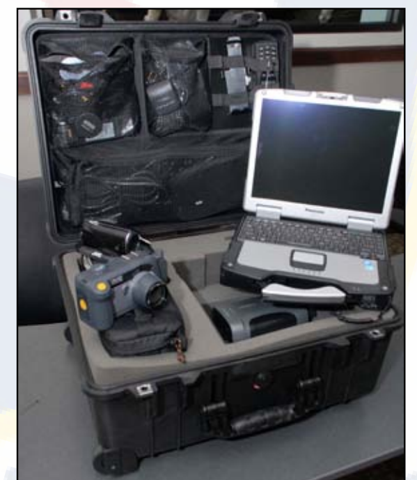
A Geospatial Information Interoperability Exploitation Portable go kit, which features self-contained communications equipment and other hardware that allow for real time and near-real time full-motion video, digital imagery and in-flight chat capability with federal, state and local emergency operations centers supporting emergency situations. (Civil Air Patrol photo by Steve Cox)
